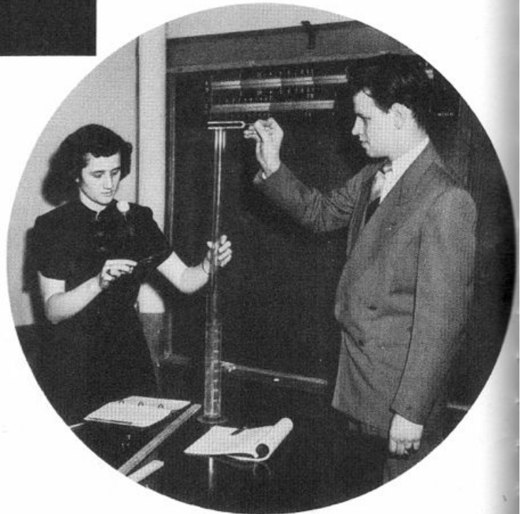
P. Kaspzyk and R. Kania spend many an hour in the Laboratory, the workshop of the individual scholar. Here they are measuring the velocity of sound.
